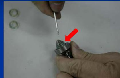
Test the tightness of Launching Rod again
