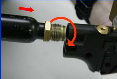
Tighten the cylinder and release the gas (switching on the valve)
