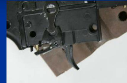
Remove the locking pin of the trigger
