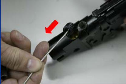
Install a screw for removal the thimble
