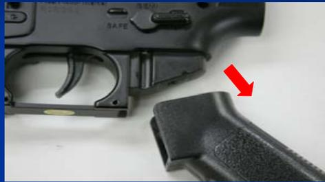
Loose the safety catch screw until the safety catch is pumped up (Safety catch should be at "SEMI" position.)
