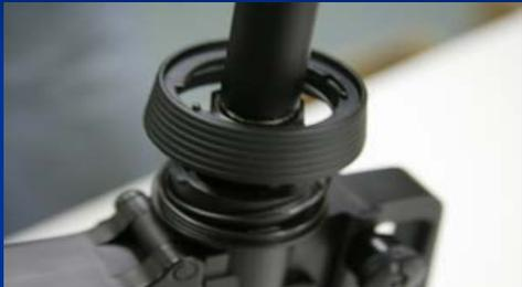
Remove the barrel lock
