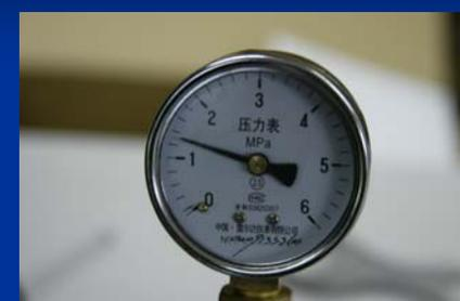
Adjust the pressure (if the needle is not pointed to 2.8MPa approximately)
