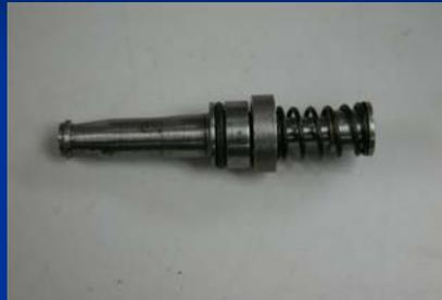
Test the tightness of Launching Rod
