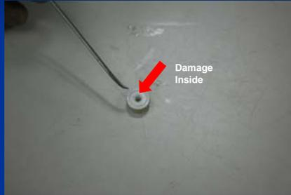
Check any damages of Valve and O-ring
