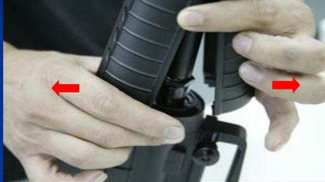
Turn the fixing ring to the proper place (shown as arrow)
