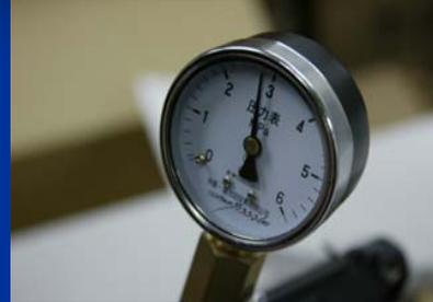
When pressure gauge shows that the needle is rising rightward, it means the gas is leaking from the pressure unit. So first of all, switch off the valve of the cylinder and release the gas in the marker core, thereafter uninstall the cylinder and pressure gauge.
