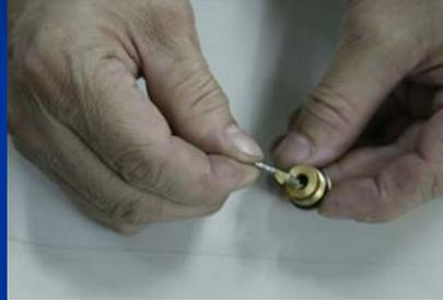
Test the valve pin smooth
