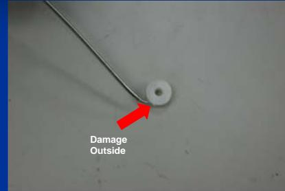
Change new Valve and O-ring and re-install all parts of the pressure unit and test the pressure again until the pressure gauge shows at 2.8MPa approximately.
