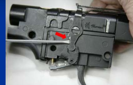
Lift up the pull bar locking sheet
