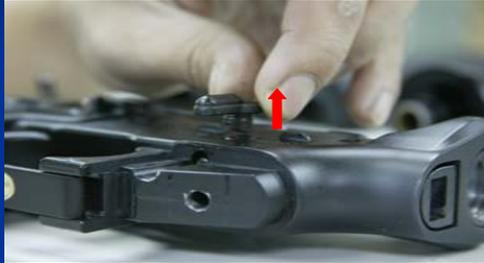
Remove the screw of magazine release catch
