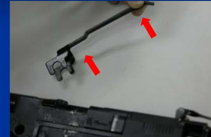
Put the pull bar locking sheet inside the chamber to connect the magnet (pointed by arrow)
