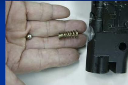
Check any damages of Valve and O-ring
