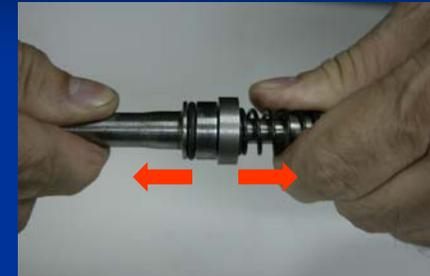
If you cannot hear any "Pop" Sound when you pull out the Launch unit, it means it is loose and necessary to change O-rings
