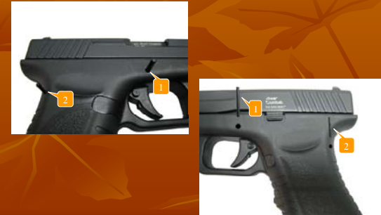
When take out the Locking Pin, keep watch for Locking Pin 1 is long & 2 is short
