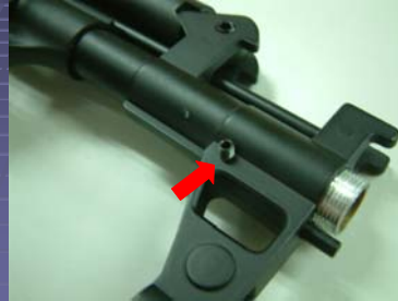
Remove the screw (on left) of the front sight
