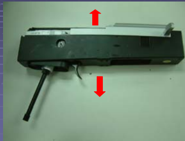
Separate the core and the lower body
