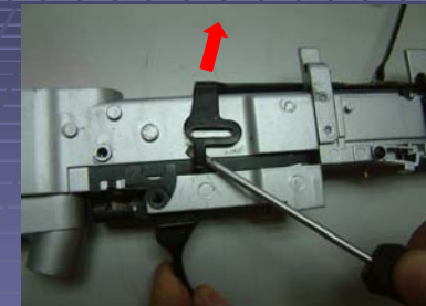
Lift up the top bar and use a tool to hold the top bar
