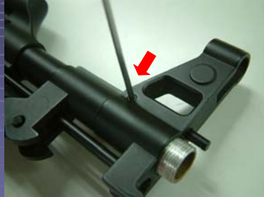
Remove the screw (on right) of the front sight
