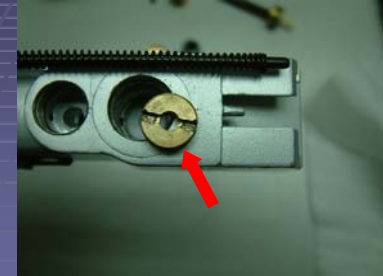
Remove the screw valve
