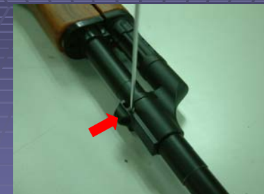
Remove the screw (on the front right) of the barrel cover
