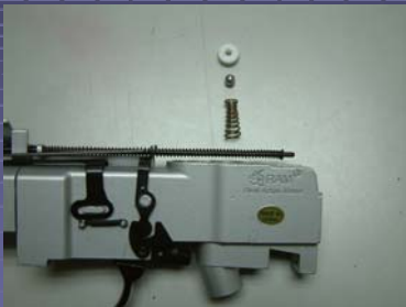
Take out the valve, spring and the steel ball
