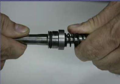
Test the tightness of Launching Rod again
