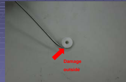
Check any damages of Valve and O-ring
