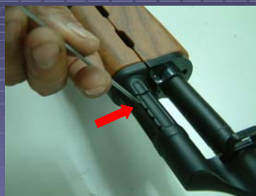
Remove the screw (on the rear left) of the barrel cover
