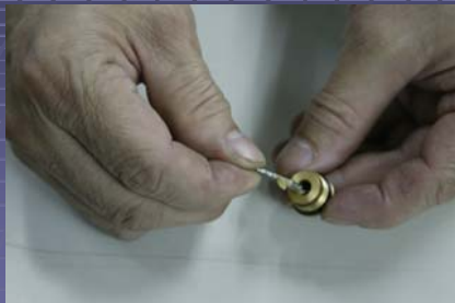
Put back the valve pin on the valve end cap
