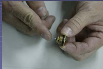
Test the valve pin smooth
