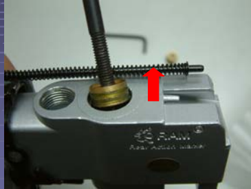
Install a screw for removal the thimble
