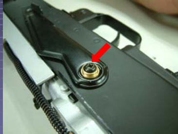
Remove the safety catch screw
