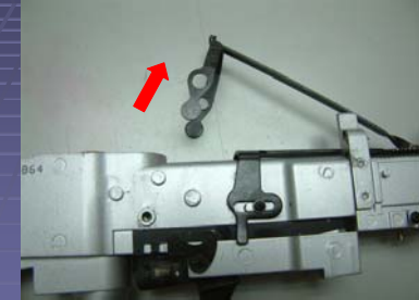
Lift up the Pull Bar Locking Sheet
