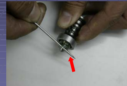
Change O-rings (supposed the Launch unit is loose)
